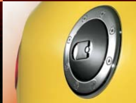
Race-style fuel filler cap trim. Manufactured in chromed ABS to avoid any fading (1M5064700).
